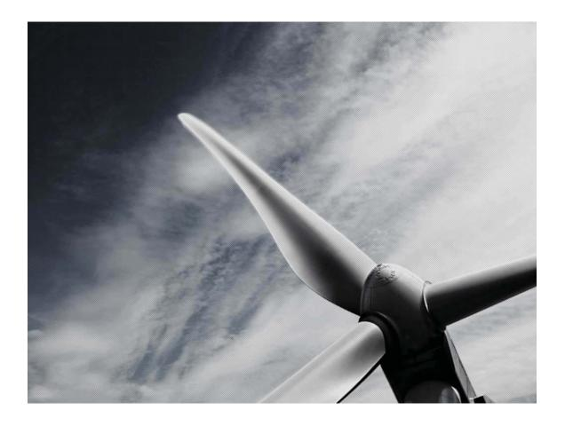
The V90 blades are about 45 metres, 150 feet, long. Each of the three are made using lightweight composite marerials to improve energy efficiency.
