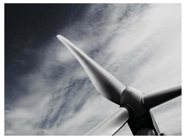
The V100 blades are about 50 metres, 164 feet, long. Each of the three are made using lightweight composite marerials to improve energy efficiency.
